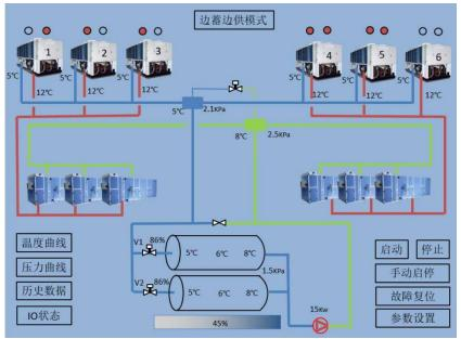
By simply utilising the excess capacity over-night from the installed chillers existing system charges the PCM tanks using conventional 5C (47F) water and later this stored energy utilised during day time to reduce the peak power demand
